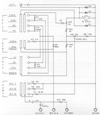
NOTE: (1) ALL RESISTANCE VALUES ARE INDICATED IN "OHM" ( $K = 10^{3}$  OHM,  $M = 10^{8}$  OHM) (2) ALL CAPACITANCE VALUES ARE INDICATED IN " $\mu$ F" ( $P = 10^{-8}\mu$ F).
