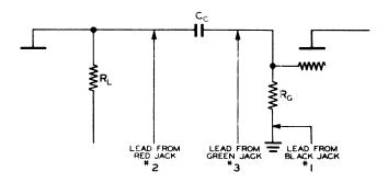
FIGURE 2. CONNECTIONS FOR MEASUREMENTS OF COUPLING CAPACITORS IN-CIRCUIT
