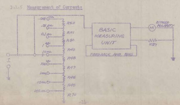
For the measurement of wheel current, a fixed multiplier
