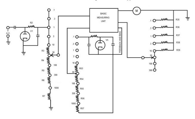
The alternating input voltage is rectified by  $V_1$  acting as a linear peak diode to produce negative direct voltage applied to the divider consisting of  $R_2$  through  $R_7$  (May be the same divider as used for d.c. voltage). This divided voltage is measured by the basic unit in a manner similar to the employed for d.c. voltage.
