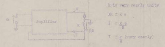
The calibration therefore depends only upon the current indication of the meter and the precision resistor R. Changes in meter resistance due to temperature (copper wound coil) and differences themselves resistance from one unit to another (in production) have no effect. It is also possible to use a multiplier R having a value smaller than the resistance of the meter, therefore providing lower full-scale ranges.
