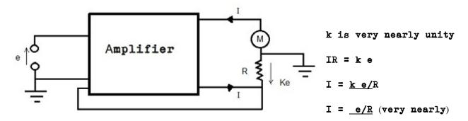
The calibration therefore depends only upon the current indication of the meter and the precision resistor R. Changes in meter resistance due to temperature (copper wound coil) and differences in meter resistance from one unit to another (in production) have no effect. It is also possible to use a multiplier R having a value smaller than the resistance of the meter, therefore providing lower full-scale ranges.
