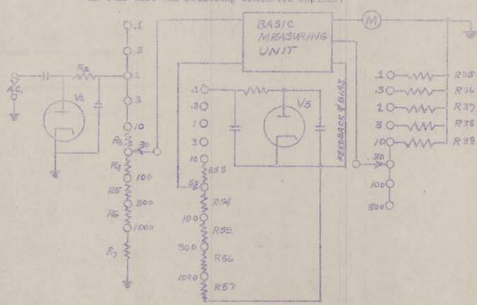
The alternating input voltage is recrified by  $V_1$  acting as a linear peak diods to produce negative direct voltage applied to the divider consisting of  $R_2$  through  $R_7$  (May be same divider as used for d.c. voltage). This divided voltage is measured by the basic unit in a manner similar to that employed for d.c. voltage.
