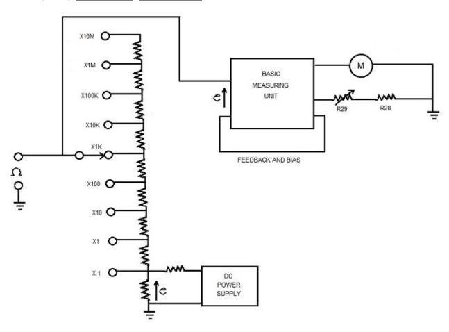
In this circuit, a stabilized d.c. power source furnished a fixed voltage E which is applied to the basic measuring unit and to the input terminals through an adjustable resistance. If the input terminals are open circuited, the voltage E is present at the input to the measuring unit and the part of the multiplier resistance  $(R_{29})$  may be adjusted to yield full scale current on the meter. If an unknown resistor is then connected, the measured voltage e is reduced according to the equation.
